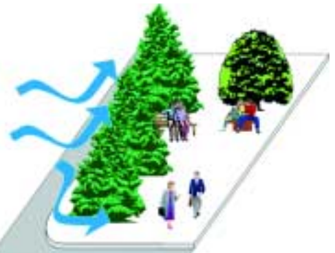
Figure 8.5: Dense canopy trees can act as wind breaks when they are placed at the prevailing wind direction in winter.
