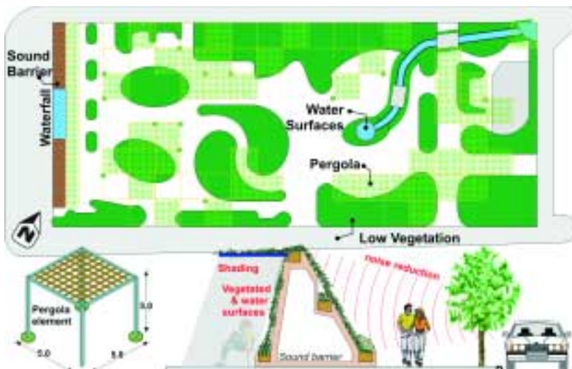
Figure 8.7: Design proposal for the site of Makedonomahon square and details of some of the proposed constructions.
