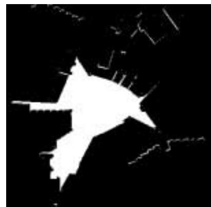
Figure 4.11: Viewshed Map. A mapping of the field of view from the middle of the site. White areas correspond to areas and surfaces within the person's potential line of sight (Matlab algorithm by Ratti [1]).
