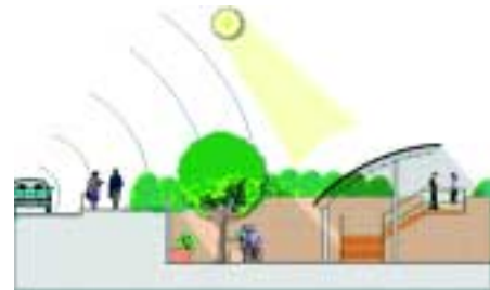
Figure 8.4: "Sunken" open spaces are an interesting solution to noise and wind protection. Tall shading devices can be easily used without interrupting the view beyond.
