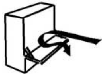
Figure 2.10: Example of counter measure for downdraft - veranda on the base of the high building.
